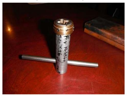
He showed a light-weight die holder he had made for cleaning threads of injector parts after silver soldering.
