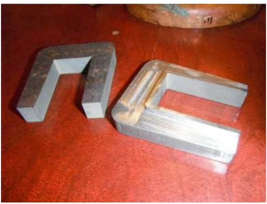
Mark Taylor showed the horn blocks made for his ride trolley which had been water cut. The back faces of the horn blocks were milled to provide a lip for mounting in
