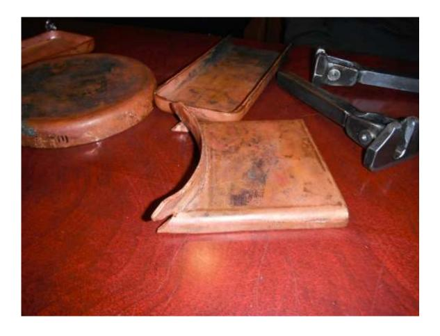
Ron Perkinson showed some of the boiler plates he had made for his Phantom boiler. Very nicely formed. He had two draw bars for the loco as well. There was discussion on marking out and drilling the tube holes in the boiler plates. The subject of easi-flo and the cost involved in fabricating the boiler was also commented on - a cause of some consternation. Ron is ready to fire up his new loco and see if heating would help un-seize the regulator valve.
