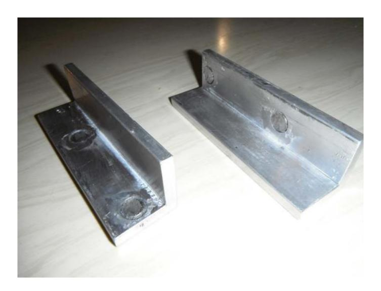
Ron Perkinson had fabricated soft jaws for his machine vice from angle alloy with small powerful magnets inset in milled cavities. A good idea and very useful.
